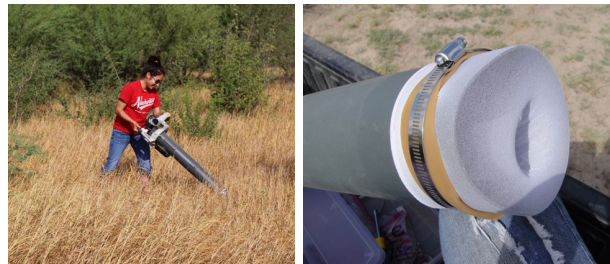
Figs. 1-2. The tick-vac in operation. The intake of the tick-vac with bag secured by hose clamp and rubber band.
